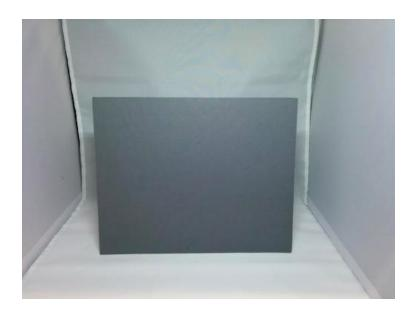
In particular, the grey card is roughly centered in the field of view, taking up around  $\frac{1}{2} \times \frac{1}{2}$  of the scene, with the white background visible on all sides around it. As is evident from the image above, a high degree of precision is not required; the most important factors are that the scene is completely static (including no light source flicker) and that the very center of the image is within the grey card area.
